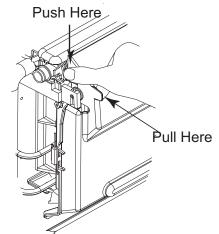
13. Remove water distributors from ice machine. Inspect distributor for restricted orifice holes. Be sure all holes are full open.
